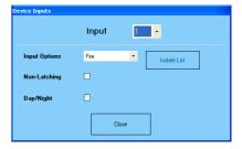
To select which input to configure, set the input number at the top of the window. For single input devices, such as detectors, this will always be set to one.
